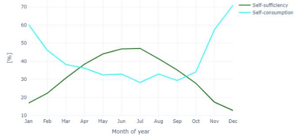
Figure 6: Monthly-integrated self-consumption and self-sufficiency for a residential PV installation in Belgium.
